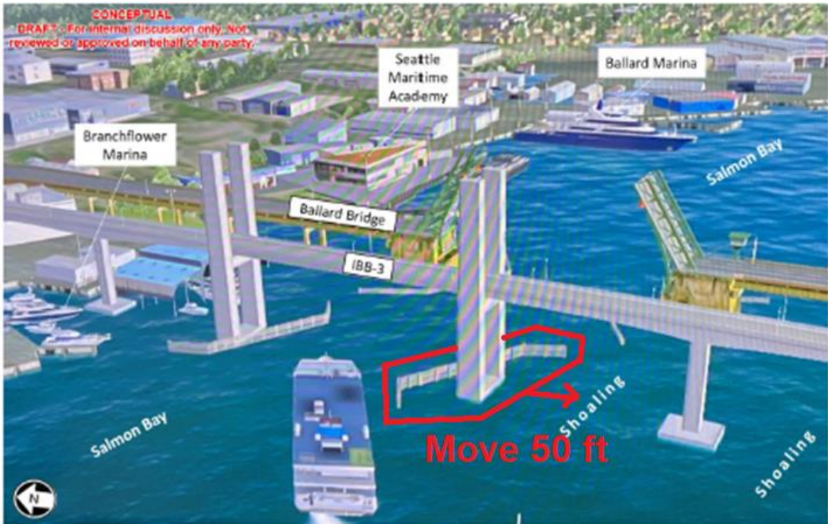
Figure 11 Reduced Turning Radius between Fishermen's Terminal and the Ship Canal Navigation Channel
