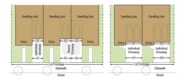
(G1+G2+G3) must be no more than 60% (D1+D2+D3) must not exceed 32 feet per frontage Individual driveway width (any "D#") shall not exceed 20 feet
